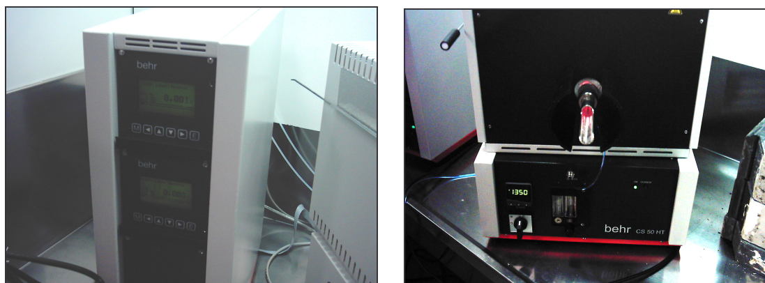
Figure 2: Detectors (left) and furnace with integrated controllers (right)
