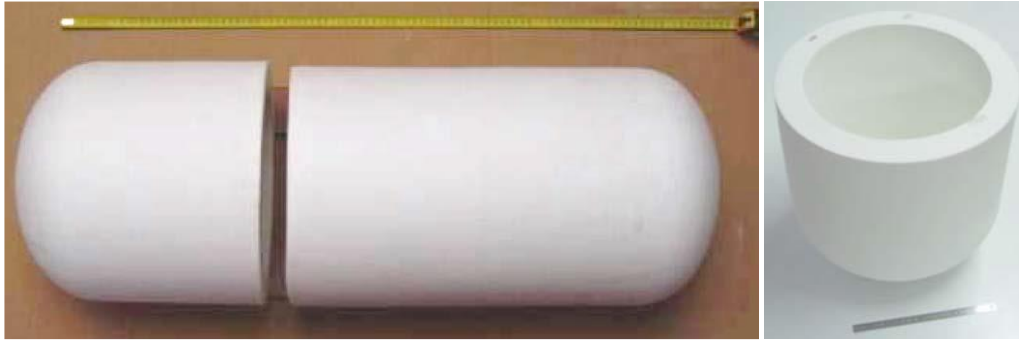
Figure 2-2: Andra half-scale model of \text{Al}_2\text{O}_3/\text{SiO}_2 VHLW canister (Baroux, 2013) (a) complete model, (b) lid.
