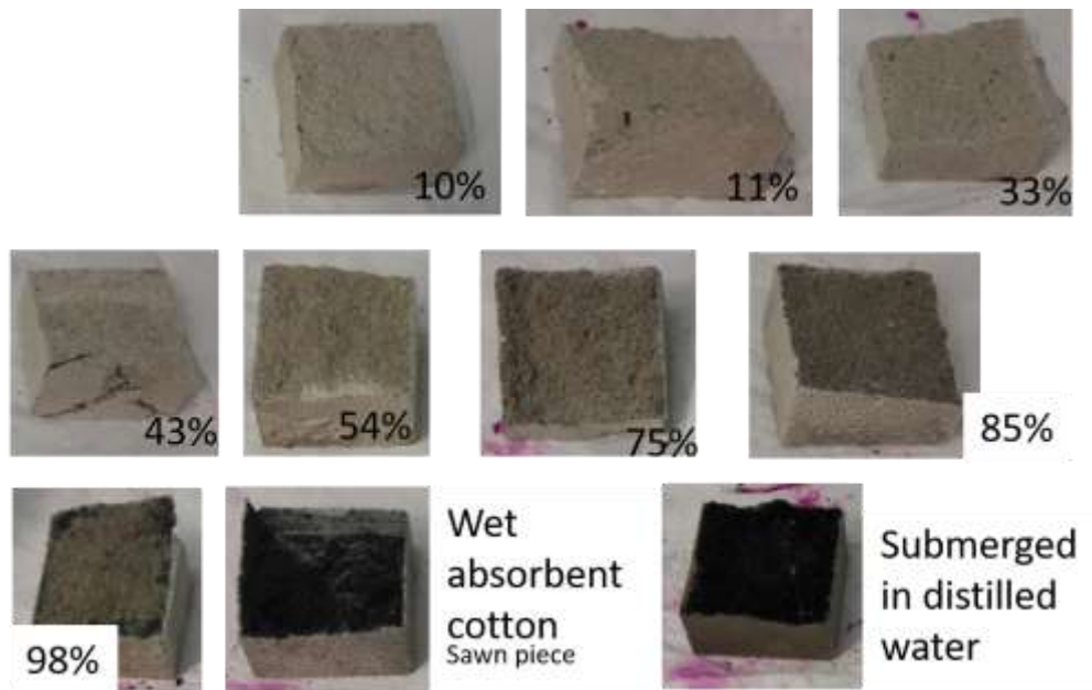
Figure 6-22: Oxidation at 20°C for backfill after 1000 days exposure to a relative humidity of cubical samples with an edge of 5 cm.
