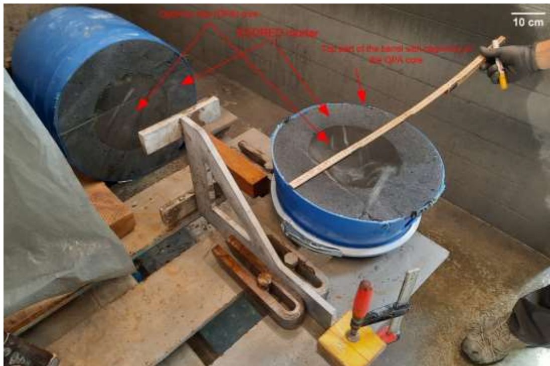
Figure 9-5: Example of slicing off of the top part of a barrel, containing only/mainly concrete/mortar, to provide access for coring/cutting specimens in the concrete/mortar volume and surrounding the Opalinus Clay (OPA) core. The barrel in this case was the one containing the interface system 2278 (ESDRED mortar/OPA interface) described below.
