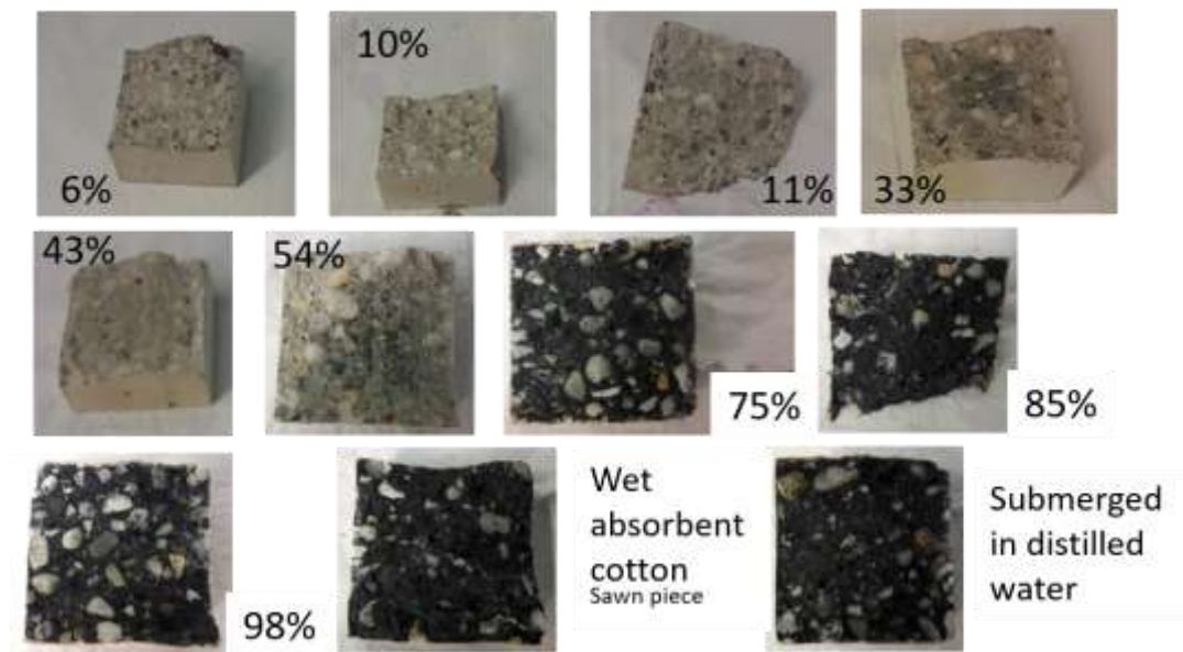
Figure 6-20: Oxidation at 20°C for buffer-like material after 1000 days exposure to a relative humidity of cubical samples with an edge of 5 cm.
