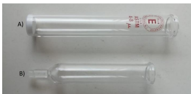
Figure 13: Two tested counter electrode chambers with each its separating porous membrane: A) porous glass frit. B) CoralPor® frit.
