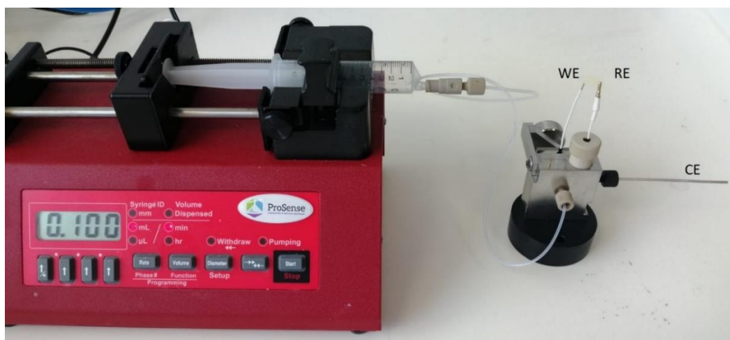
Figure 15: Flow cell experiment setup, with the syringe pump containing the syringe and the assembled radial flow cell.
