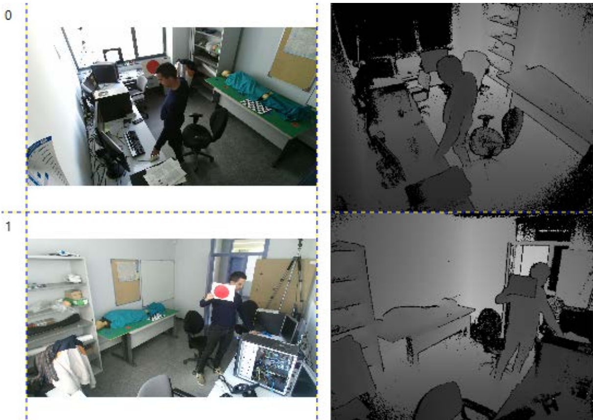
Figure 11. Camera calibration: both cameras must see the selected pattern
