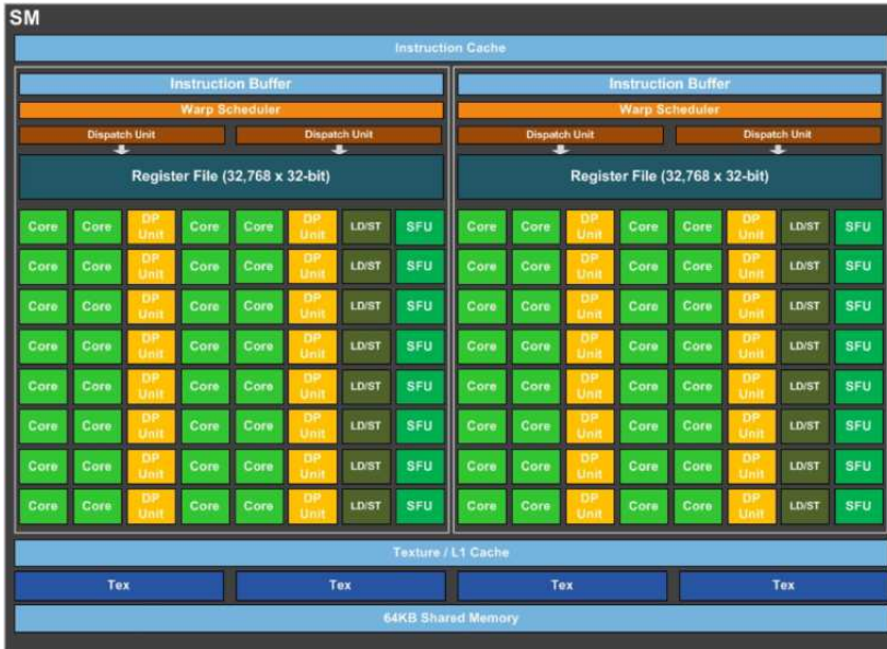
Figure 5.4: Streaming Multiprocessor of the Pascal architecture [63].
