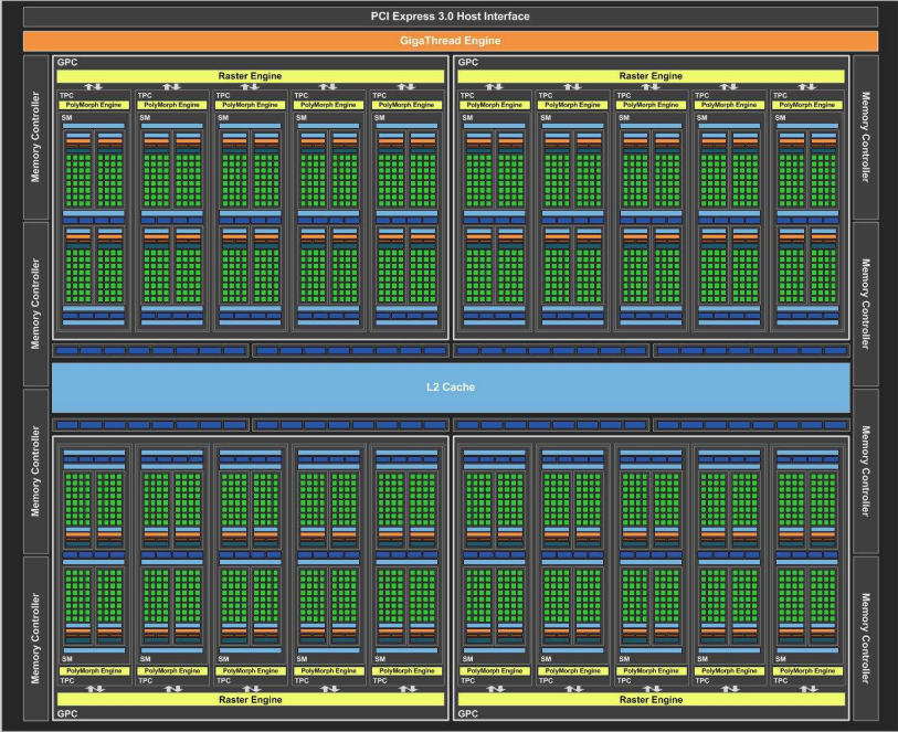
Figure 5.3: The GP104 chip based on Pascal architecture [63].
