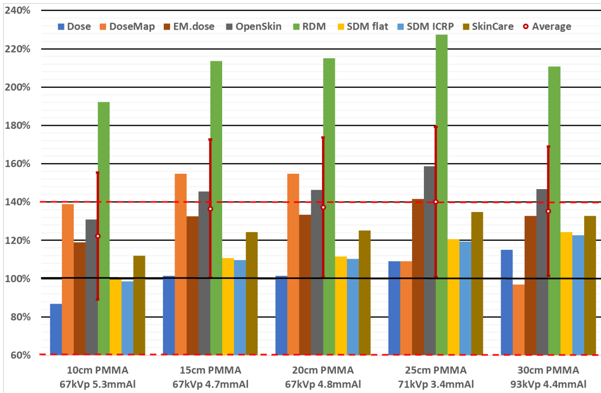
Figure 5: MSD estimated using SDC software tools for PMMA thicknesses ranging from 10 to 30 cm on a GE Innova IGS 540 system; MSD estimates are normalised to measured doses. Tube voltage (kVp) and HVL values (mmAl) of the irradiation are reported on the second line of the horizontal axis. Red horizontal bars represents the \pm 40\% deviation range as per the acceptability criteria of the Acceptance protocol; the COV is represented as error bars drawn from the average MSD estimate.
