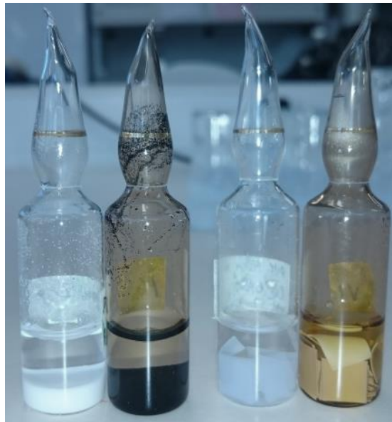
Figure 1: The effect of radiation on the appearance of PVC materials. Imaged are flame-sealed vials containing saturated \text{Ca}(\text{OH})_2 and (from left to right) non-irradiated PVC powder; irradiated PVC powder; non-irradiated PVC sheet; irradiated PVC sheet. Note the change in colour of the PVC powder from white to black, and of the PVC sheet from clear translucent to light brown opaque.
