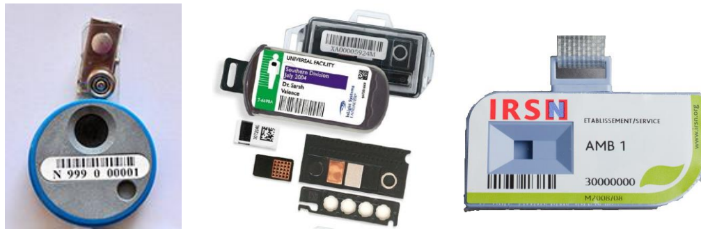
Figure 1. TL (left) [3], OSL (center) dosimeters from Landauer [4] and RPL (right) dosimeter from IRSN [5].
