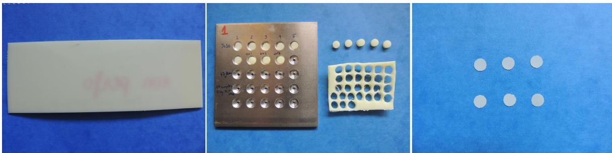
Figure 4 - Efficast material before being coated (left), punched samples with \text{Al}_2\text{O}_3:\text{C},\text{Mg} coating (middle) and punched RPL paper samples (right)
