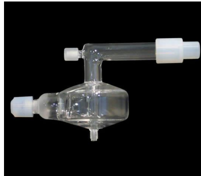
Figuur 1. Cyclonic spray chamber (Elemental Scientific, 1999)
