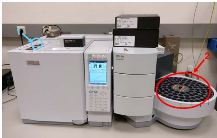
Figure 13. Gas Chromatograph used for the determination/separation of ^{14}\text{C} gases produced from corrosion experiments. (1) Manual injection and (2) Auto sampling.
