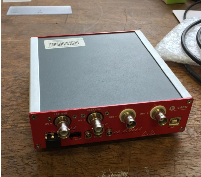
Figure 2.5 – The CAEN DT5780 acquisition system.
