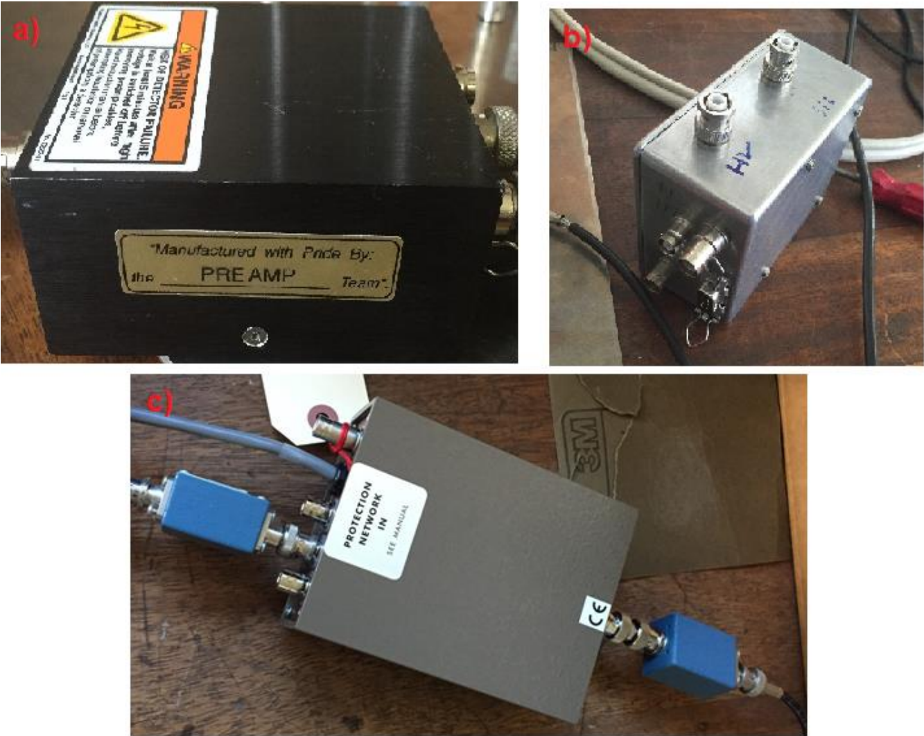
Figure 3.1 - Picture and scheme of the three preamplifiers. a) Canberra preamp, b) SCK preamp, c) Ortec preamp.
