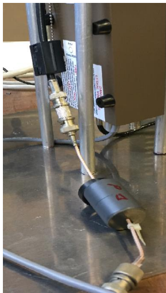
Figure 3.8 – Spikes remover magnetic filter.
