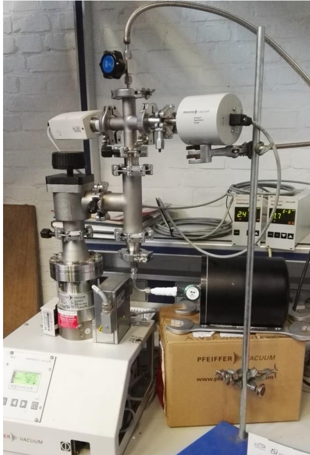
Figure 1.6 – The vacuum and gas handling system.
