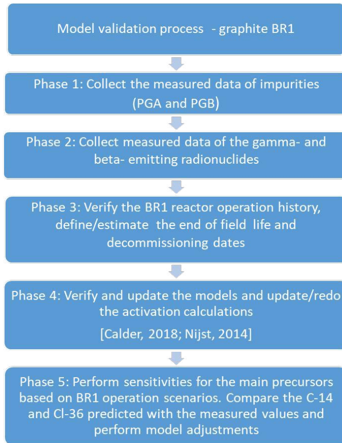
Figure 2. Flow chart showing the steps or phases of the modelling validation process.
