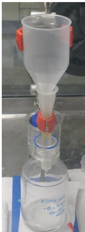
Figure 2. Image taken from the set-up used for securing the chromatographic column during the various steps of Am(III)/Pu(IV) separation
