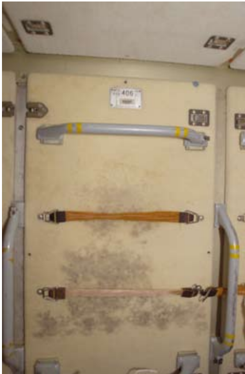
Figure 3: An example of microbial contamination that developed on an interior panel aboard the ISS. Attempts to clean the panel with supplies aboard the ISS failed and the panel had to be replaced. (Credit: NASA, image ISS010E11563)
