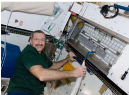
Figure 1: NASA astronaut Dan Burbank cleans cabin air bacteria filters in the Tranquillity node of the ISS (Credit: NASA)
